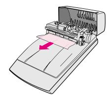
4 If you still cannot remove the paper from the ADF, lift the ADF lid to its fully open position, loosen the jammed paper from the roller at the rear of the ADF lid, and pull it gently from the ADF.
